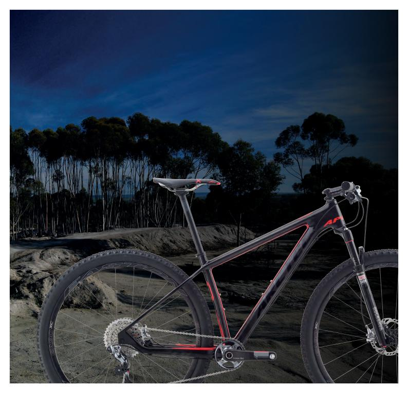
**TAPERED HEAD TUBES** increase the contact area between the fork crown and the head tube and increase rigidity. This increases the responsiveness and feeling of agility in the front end of the bike.
